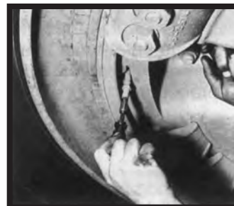
Removing valve core from single piece wheel.
