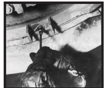
Running wire through the stem of an single piece wheel.
